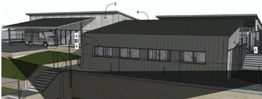
2. Fibre cement facade panels EQUITONE tectiva or similar Colour TE90 Calico
